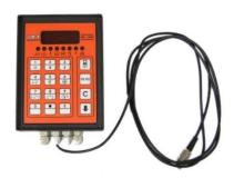
Error messages are displayed as codes. All possible codes are described in the following summary. Once an error code is displayed, for example "E13", the display can be cleared by pressing the down arrow twice.
